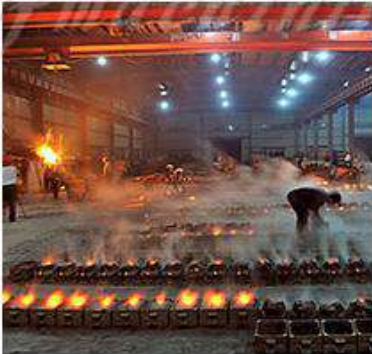
5 pouring and making sand core
